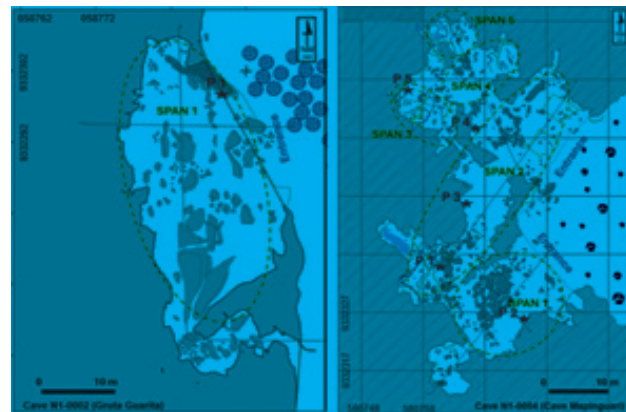
Figure 2 : Topographic maps of Caves N1-0002 and N1-0004 showing the spans and unstable points (blue stars)
