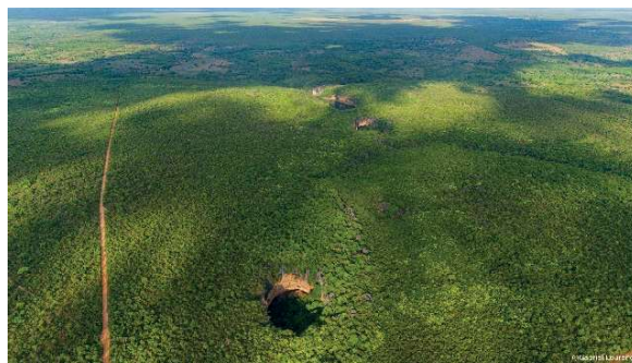
Figure 1: Collapse sinkholes with limestone cliffs, aligned in the ENE-WSW direction, parallel to a major cave system. The low gradient landscape that surrounds the sinkholes is covered by sandstone. The major axis of the sinkhole in the foreground is 180 m, and its depth is 90 m. Photo: Gabriel Lourenço.
