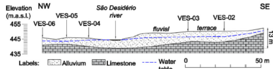
Fig. 7. Geological interpretation of the São Desidério River geophysical cross-section. The erosive contact between the alluvium deposits and the limestone rock is represented. The locations of the vertical electrical soundings are indicated as “VES”. Note the maximum sediment thickness of 13 m from the top of the river terraces to the lowest limestone erosive surface elevation. A reference station at the profile was tied to GNSS positioning data for a more precise elevation representation.
